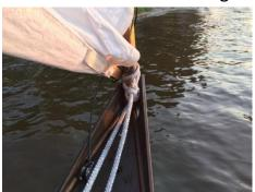
Tighten the yard at the bow, by pulling tack line, which then fixed in rear cockpit.
